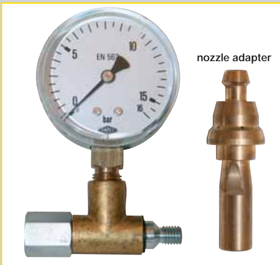
Pressure control device 0-16 bar for cutting oxygen for torch head assembly. For pressure monitoring the corresponding cutting nozzle will be screwed into the outlet. For use with BGB nozzle mix add on nozzle adapter. Art. No. 0004457010
